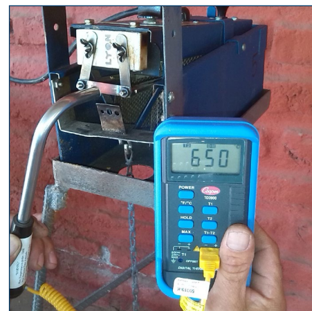
Pyrometer indicating proper blade temperature of 650°C.
